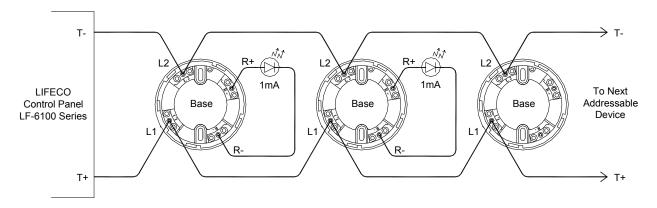
The detector circuit requires a twisted pair copper cable with a diameter of not less than  $1.5 \text{mm}^2$ . The total resistance of the conductor based on the loop length should not exceed  $30\Omega$ .
