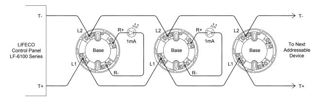
The detector circuit requires a twisted pair copper cable with a diameter of not less than 1.5mm<sup>2</sup>. The total resistance of the conductor based on the loop length should not exceed  $30\Omega$ .
