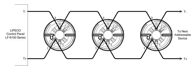
The detector circuit requires a twisted pair copper cable with a diameter of not less than  $1.5 \text{mm}^2$ . The total resistance of the conductor based on the loop length should not exceed  $30\Omega$ .
