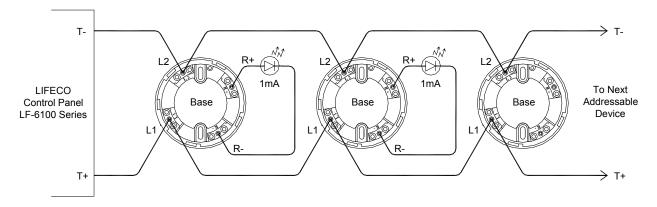
The detector circuit requires a shielded twisted pair stranded copper cable with a diameter of not less than 1.5mm<sup>2</sup>. The total resistance of the conductor based on the loop length should not exceed  $30\Omega$ .
