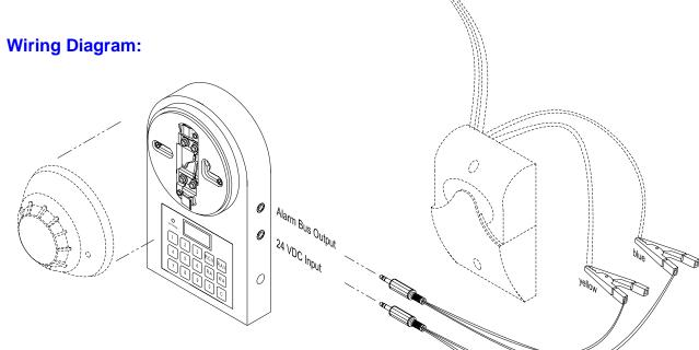
The LF-DP-6190 Address Programmer can be used either by installing a detector through its fascia or through alligator clips depending on the type of bus equipment. The first set socket terminal on the right side (yellow, blue lines) is the Alarm Bus Output Line which is used for address coding and analog value operation reading. The second set socket terminal (red, Black lines) is 24 V Power Supply Input Line which is used when the programmer uses external power supply.
